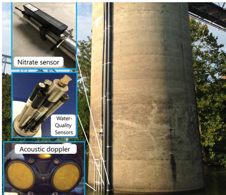
Photo of the super gage located on the Ohio River at Ironton, OH with insert photos of the water-quality and streamflow equipment. Photo courtesy USGS.
