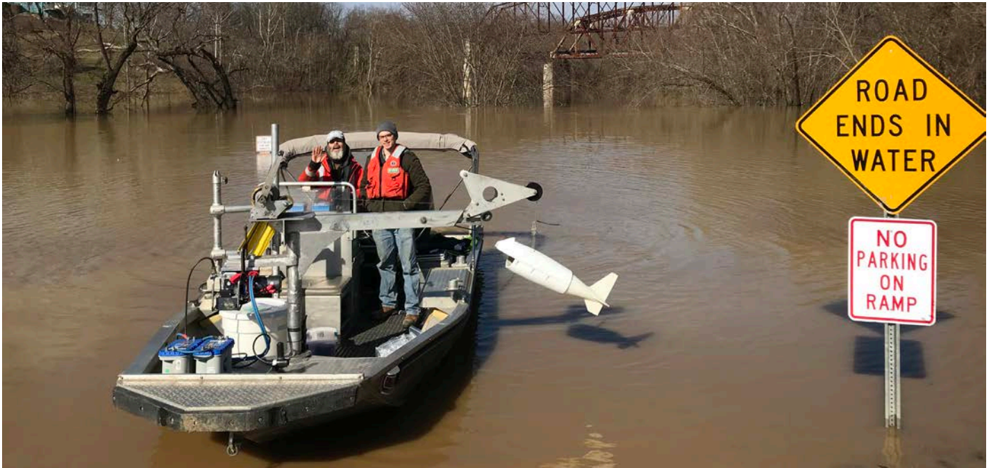
USGS crew finishing collecting a discrete representative water-quality sample for the super gage on the Licking River at Highway 536 near Alexandria, KY.
